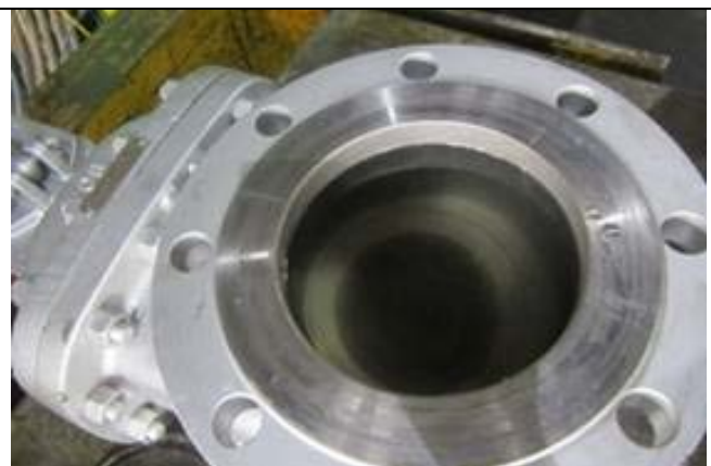
Leakage check during low pressure closure test
