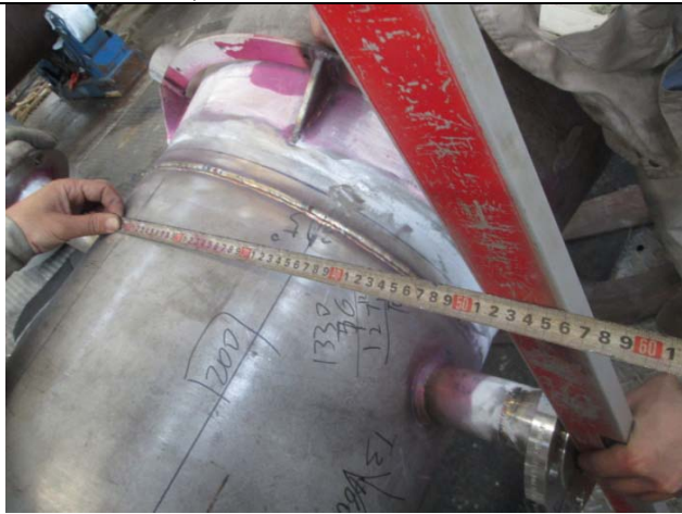
Photo 23: Location check of nozzle L2 (Out of the tolerance )
