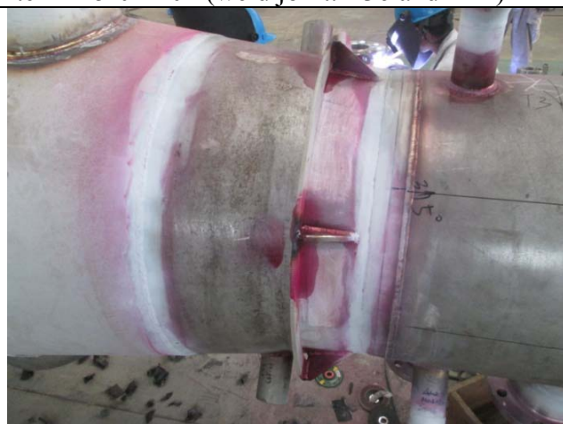
Photo 32: LPT of seam of skirt with head of item 445-01-204 (weld joint: E36 and FB1)
