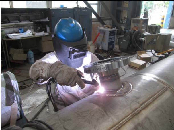
Photo 5: Welding materials traceability check for ER308L
