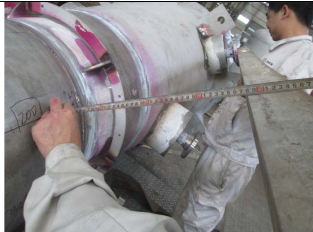
Photo 26: Location check of nozzle B3 (Out of the tolerance )
