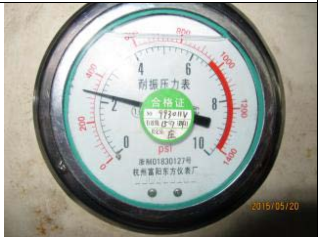
Showing the test pressure for 2" 150Lb;
