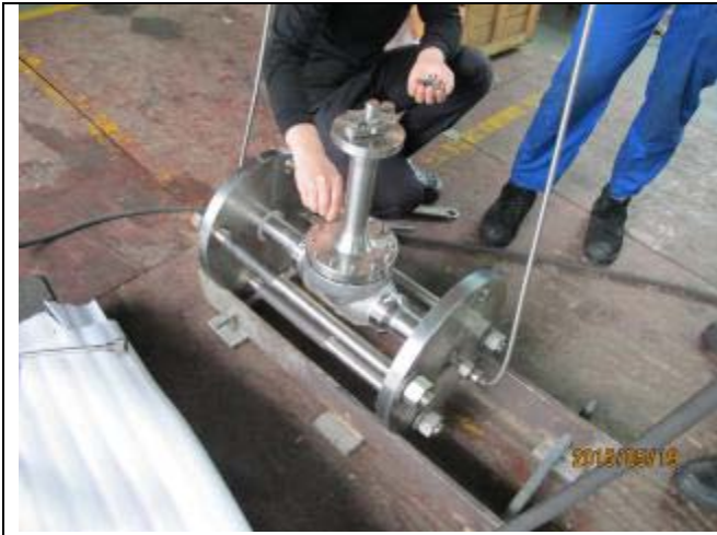
Showing assembling valve 2" 150LB;
