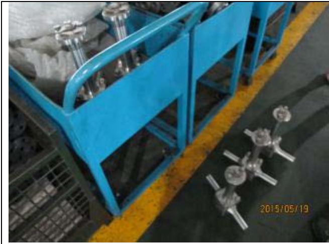
Showing the finished valves; 1" 800lb
