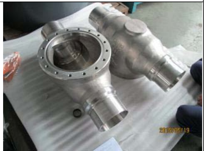
Showing the valves waiting for assembling; 6" 150LB
