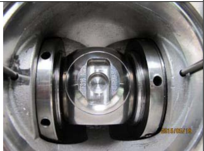
Showing the inside condition clean and no oil;
