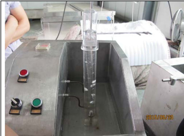
Showing the leakage for 2" 150Lb;
