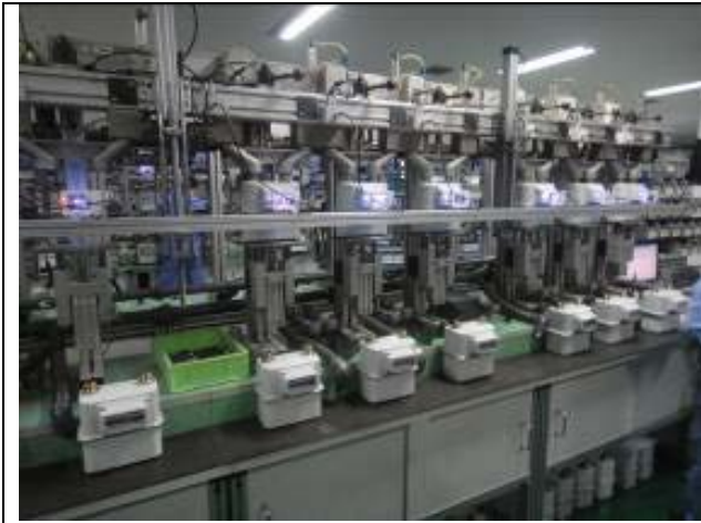
calibration and pressure absorption testing
