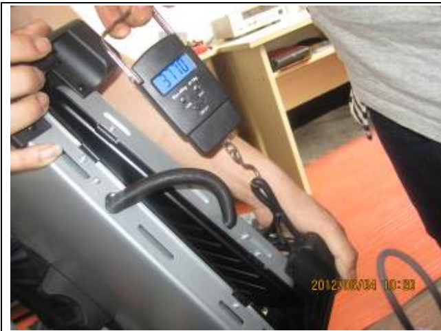
Cable pull test
