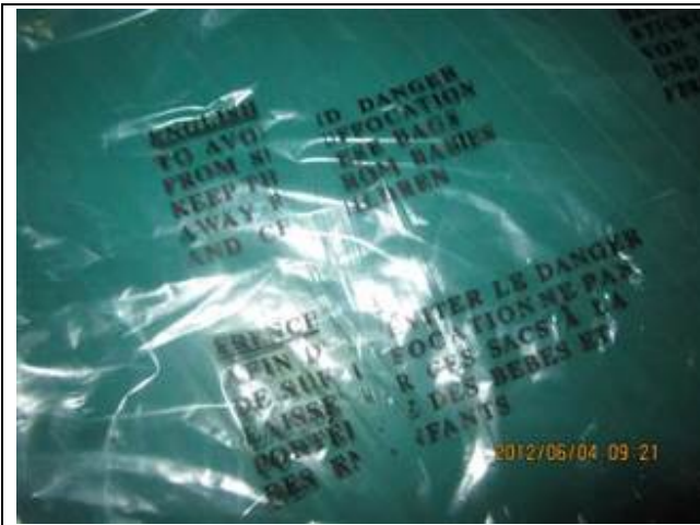
Defect - the marking on poly bag poor printed
